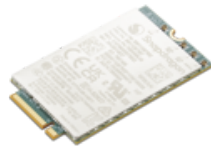
ThinkPad Foxconn SDX61 5G Sub6 PCIE M.2 3052 WWAN module for T14 G7
