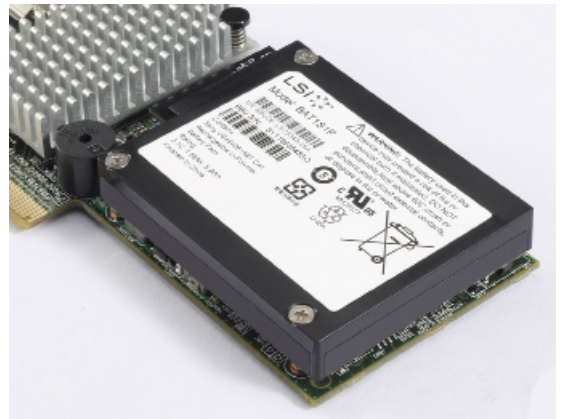
ThinkServer RAID 700 Adapter with battery (LSI SAS 9260-8i with iBBU08)
